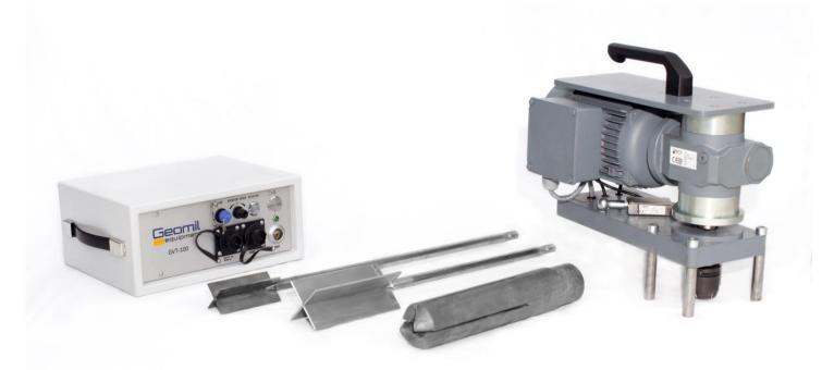
The Geomil Equipment GVT-100 field vane tester is a sophisticated PLC controlled device with a high precision torque sensor. The testing procedure and data acquisition are fully software controlled.
