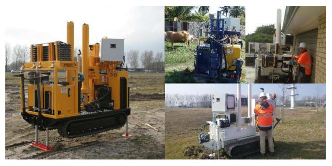
The Geomil Equipment Lynx-200 is a compact and versatile self-propelled unit, specifically designed for Cone Penetration Testing (CPT) in confined or difficult to access areas where larger and fully ballasted rigs cannot be deployed.
