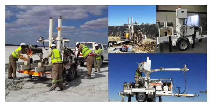
The Geomil Equipment Husky-200 is a trailer mounted Cone Penetration Testing (CPT) system, providing a high quality design with simple operating features. The Husky is an affordable solution and aimed at operators that frequently need to conduct CPT's.
