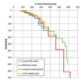
S-wave velocity curves calculated from dispersion curves for multiple sites in New Orleans.
