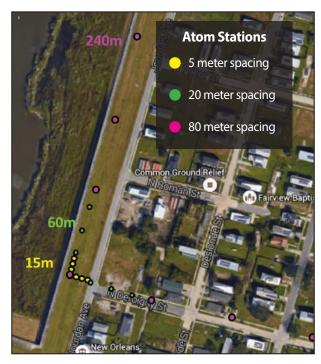
L-shaped array in the Lower 9th Ward, New Orleans, using the Atom Passive Seismic System.
